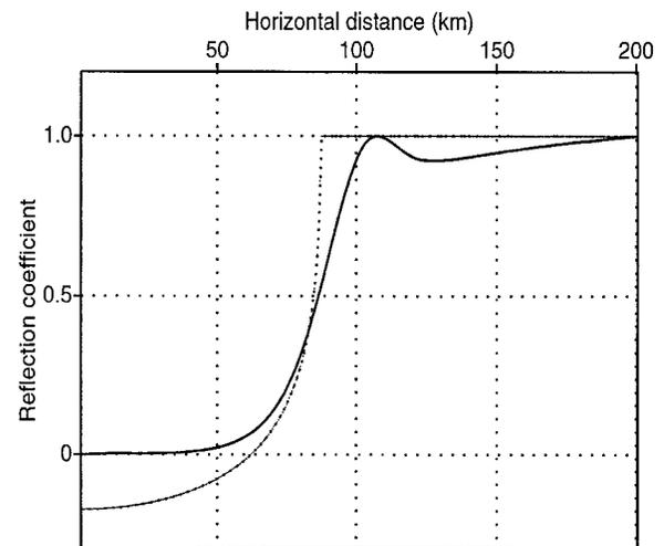
Figure 1. Comparison of reflection coefficients between theoretical (dotted line) and the calculated one by screen method (solid line).
