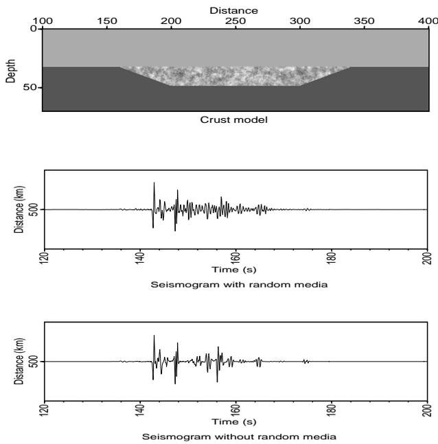
Figure 14. A heterogeneous crustal model representing a mountain root with small-scale random heterogeneities (top panel). The comparison between synthetic seismograms with and without random heterogeneities are shown on the middle and bottom panels, respectively.
