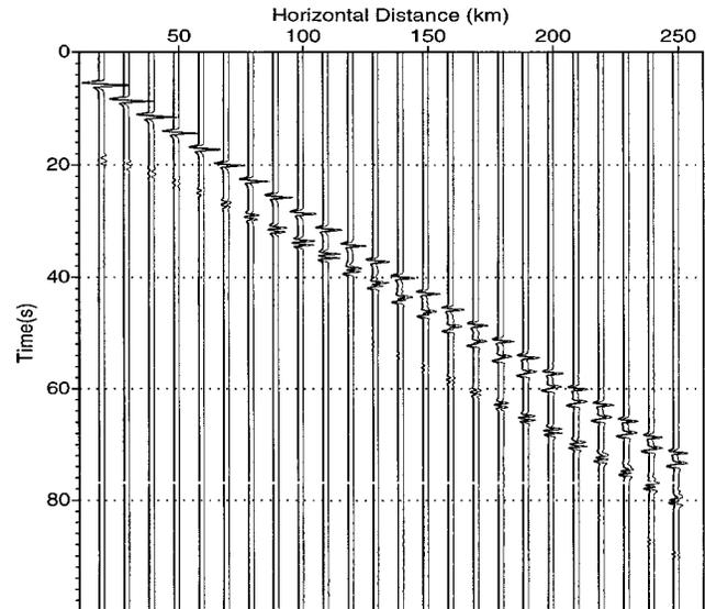
Figure 5. Comparison of synthetic seismograms along the surface calculated by the screen method (thick lines) and reflectivity method (thin lines) for a flat crustal model (32 km thick). The source function is a Ricker wavelet with dominant frequency of 1.0 Hz.
