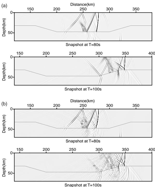
Figure 15. Comparison between snapshots for waves passing through a 'mountain root' (a) with or (b) without random heterogeneities.
