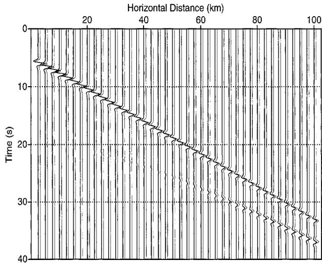
Figure 2. Comparison of synthetic seismograms between the screen method and the fourth-order finite difference method for Moho reflection without free surface. The source function is a Gaussian derivative. The first and second arrivals are the direct and reflected waves, respectively.
