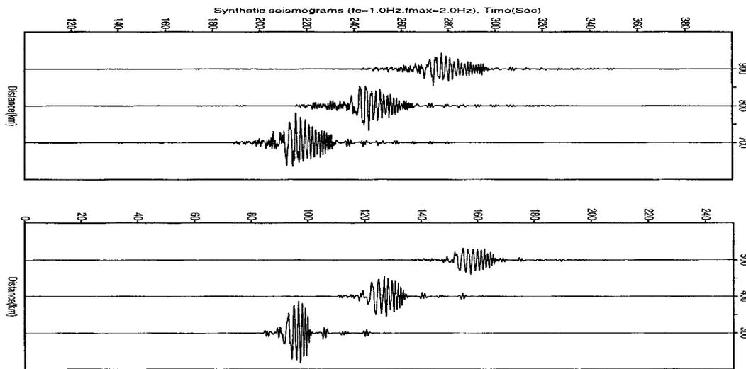
Figure 13. Low-frequency ( $f_c = 1$  Hz,  $f_{\max} = 2$  Hz) synthetic seismograms on the surface at distances up to 1000 km for an inhomogeneous crustal waveguide.
