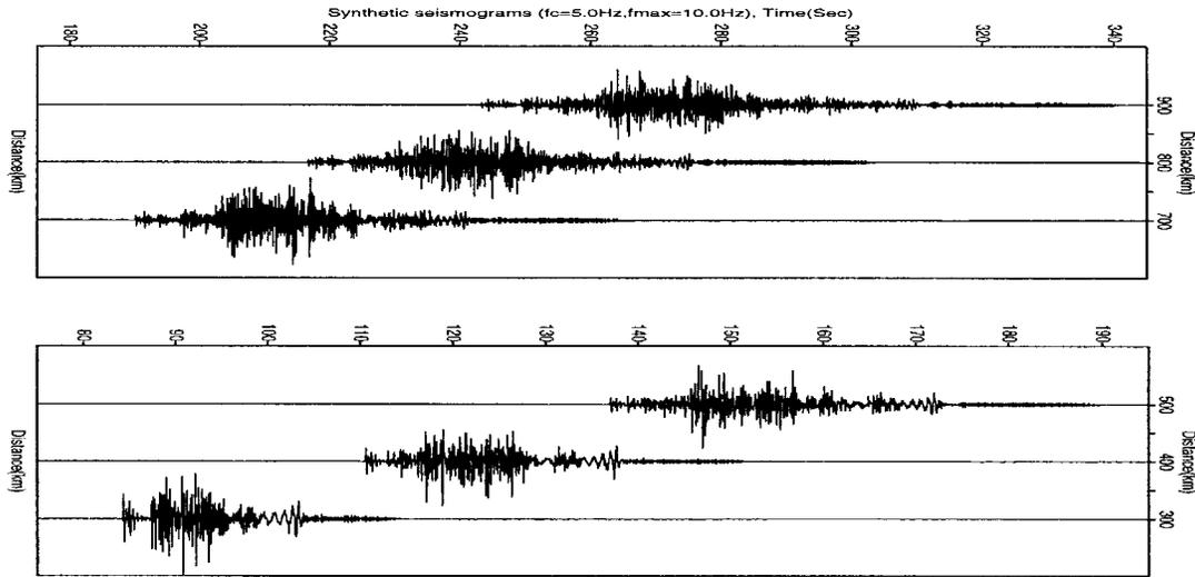
Figure 12. High-frequency ( $f_c = 5$  Hz,  $f_{\max} = 10$  Hz) synthetic seismograms on the surface at distances up to 1000 km for an inhomogeneous crustal waveguide.
