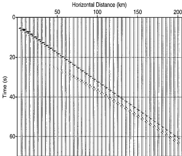
Figure 4. Comparison of reflection seismograms using small- and wide-angle screen propagators. The reference velocity and density used in calculation are 2.9 km/sec and 2.7 g/cm<sup>3</sup>. The parameters of the crust and the mantle are the same as the previous examples.
