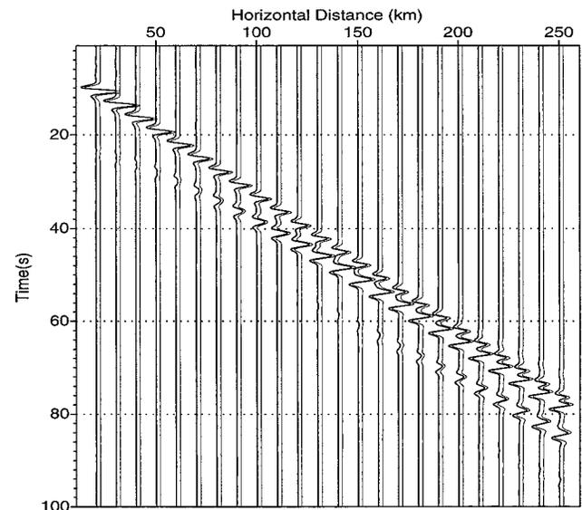
Figure 6. Comparison of synthetic seismograms along the surface calculated by the screen method (thick lines) and the fourth-order finite difference method (thin lines) for a flat crustal model (32 km thick). The source function is a Gaussian derivative ( $f_0 \sim 0.5$  Hz).
