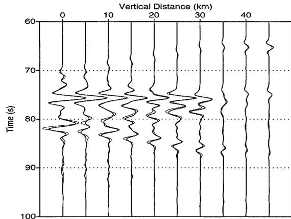
Figure 7. Comparison of synthetic seismograms along a vertical profile at the distance of 250 km calculated by the screen method (thick lines) and a finite difference method (thin lines) for a laterally varying crustal model shown on the top panel.
