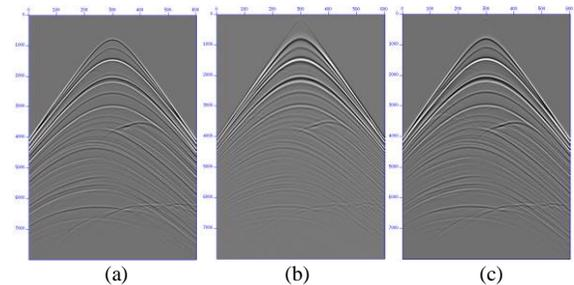
Figure 3 seismic data(a), demigration data with RTM result(b), demigration data with LSRTM result(c).
