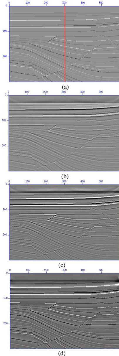
Figure 1. true reflectivity model (a), conventional RTM result (b), RTM with the use of RI propagator (c) and LSRTM result with the use of RI propagator (d)
