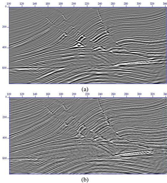
Figure 4. RTM result (a) and LSRTM result (b)
