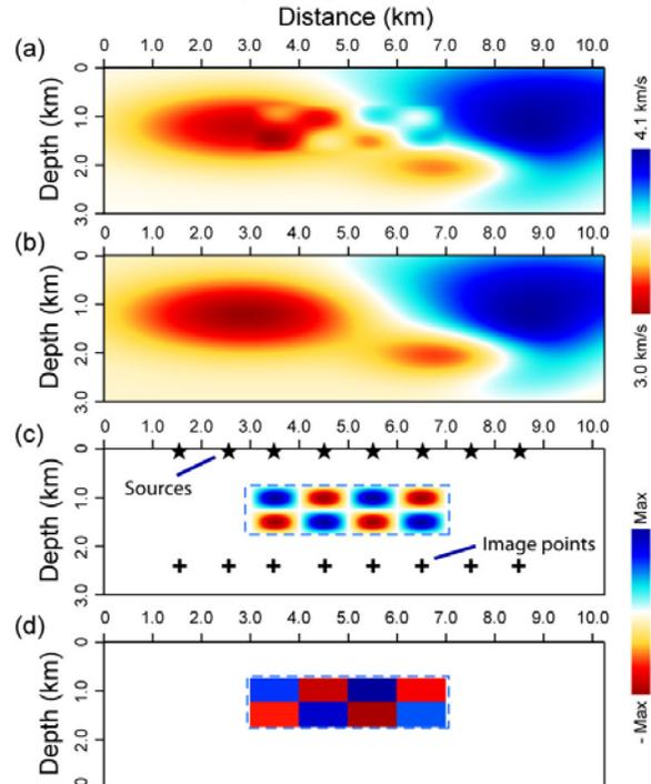
Figure 4. Inversion for variable background model, with (a) true velocity model, (b) background velocity model, (c) velocity perturbation, and (d) inverted perturbation.
