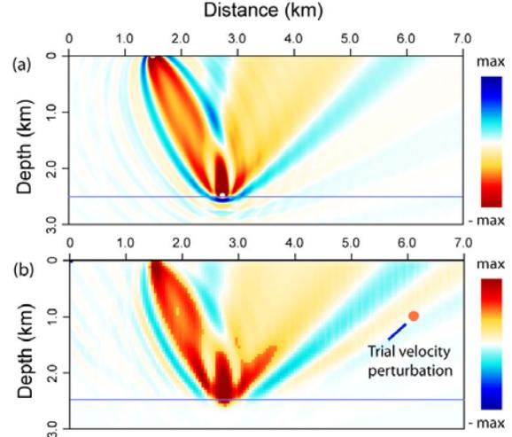
Figure 1. A sensitivity kernel for a shot gather image, with (a) theoretical sensitivity kernel, and (b) the sensitivity map directly measured from migration imaging.
