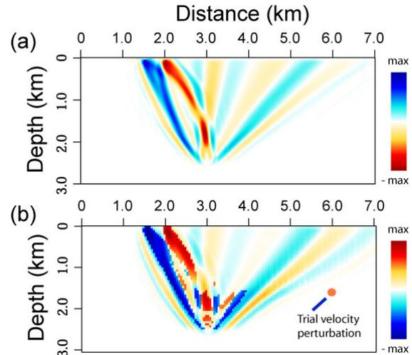
Figure 2. A broadband differential sensitivity kernel for a variable background velocity model, with (a) the theoretical kernel, and (b) directly measured sensitivity map for RMO.
