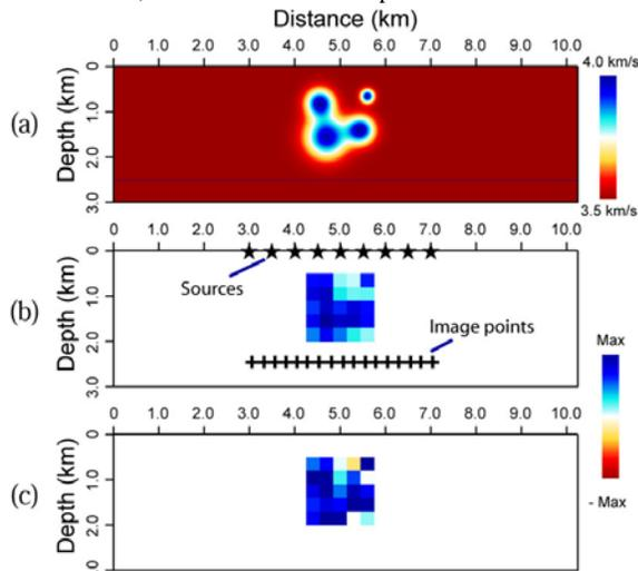
Figure 3. Inversion for constant background velocity model, with (a) true velocity model, (b) discretized velocity perturbation, and (c) inverted perturbations.
