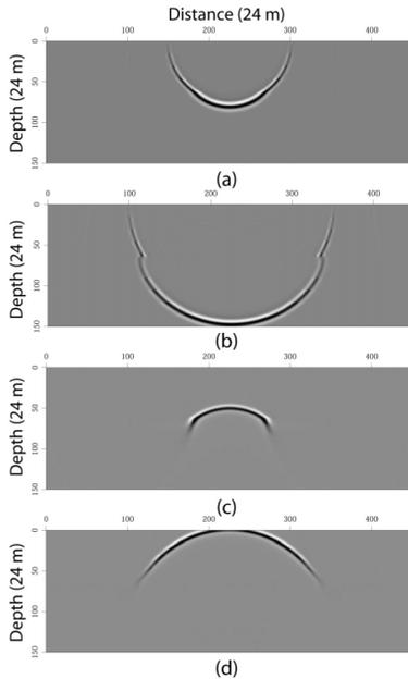
Figure 3. Wavefield snapshots reconstructed using the one-way propagator. (a) and (b) are wavefields along  $+z$  and at 0.8 s and 1.2 s. (c) and (d) are wavefields along  $-z$  and at  $T-0.8$ s and  $T-1.2$ s. Note that compared with the finite-difference result shown in Figure 2, the undesired reflections have been eliminated.
