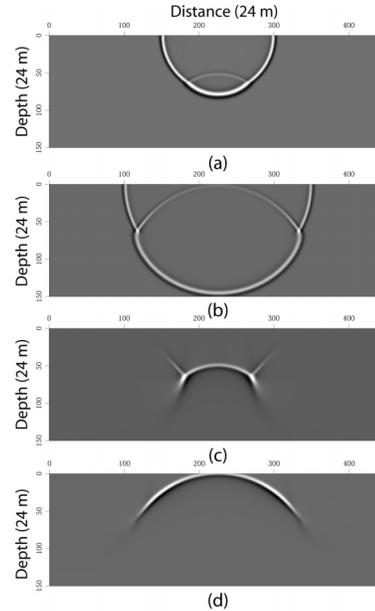
Figure 2. Wavefield snapshots calculated using full-wave finite-difference method. (a) and (b) are source wavefields at 0.8 s and 1.2 s. (c) and (d) are receiver wavefields at  $T - 0.8$ s and  $T - 1.2$ s.
