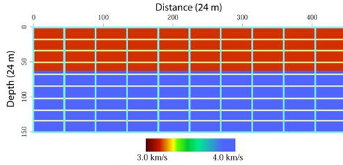
Figure 1. A simple two-layer velocity model. The horizontal and vertical lines indicate the locations where wavefields are needed for one-way extrapolations.
