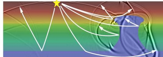
Figure 5. A simple salt dome model with steep flanks. Overlapped is the snapshot generated by finite-difference forward modeling. The major reflection events are marked with rays.
