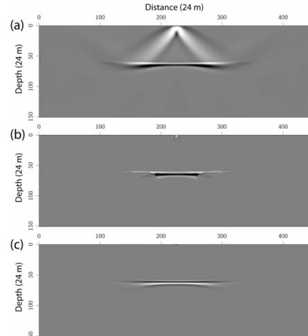
Figure 4. Reverse-time images for the two-layer model, (a) using conventional zero-lag image condition, (b) using the image condition given by Yoon et al. (2004), and (c) using full-wave propagator plus local one-way propagator.
