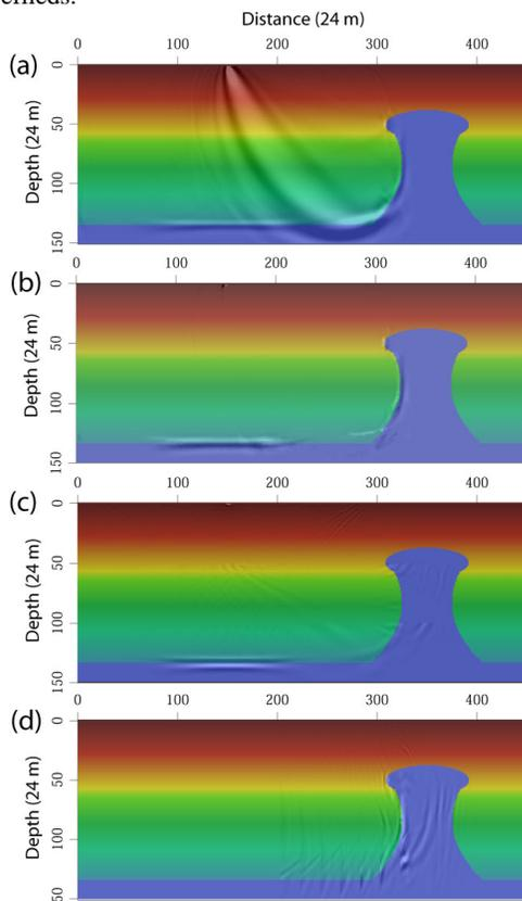
Figure 6. Depth migration image for a simple sand dome model, (a) using the conventional zero-lag imaging condition, (b) using the image condition of Yoon et al. (2004), (c) using  $u_s^{+z}(\mathbf{r})u_g^{-z}(\mathbf{r})$  and (d) using  $u_s^{+x}(\mathbf{r})u_g^{-x}(\mathbf{r})$ .
