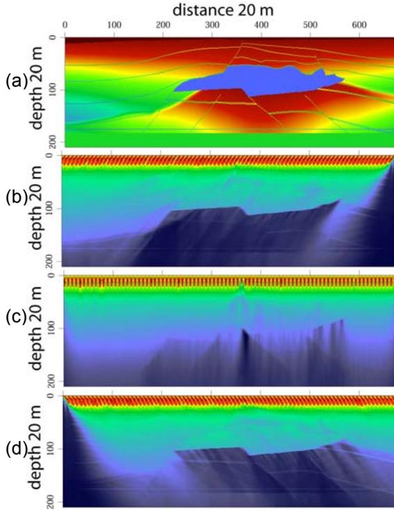
Figure 3. DI maps for the 3D SEG/EAGE salt model. Shown in the figure are cross sections at  $y = 6100$  m, with (a) velocity model, (b) DI of  $45^\circ$  left, (c) vertical DI, and (d) DI of  $45^\circ$  right.
