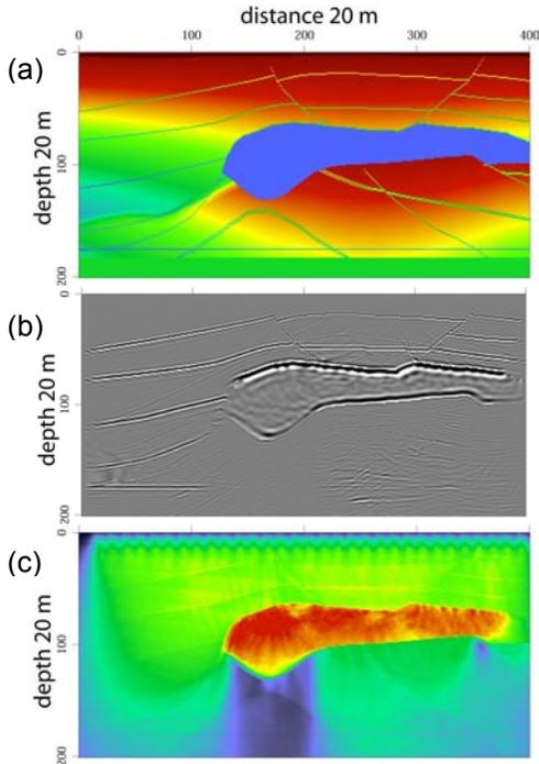
Figure 5. ADRs for the 3D SEG/EAGE salt model. Shown in the figure are cross sections at  $y = 2440$  m, with (a) velocity model, (b) prestack depth image and (c) vertical ADR.
