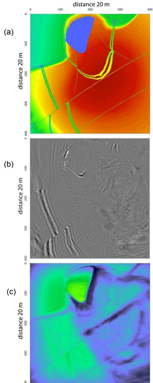
Figure 6. ADRs for the 3D SEG/EAGE salt model. Shown in the figure are depth slices at  $z = 2500$  m, with (a) velocity model, (b) prestack depth image and (c) total ADR.
