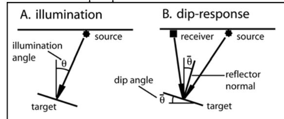
Figure 2. A sketch showing (a) the directional illumination and (b) the acquisition dip-response.
