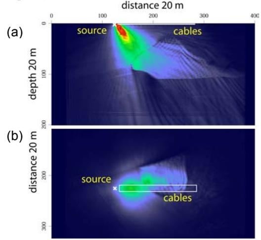
Figure 4. The ADR from a single shot in a 3D model. The dip angle is  $30^\circ$ . Shown in (a) is the vertical profile, (b) is the depth slice at  $z = 1000$  m. The acquisition system composed of a source and four 3200 m cables, which have been marked in the figure.
