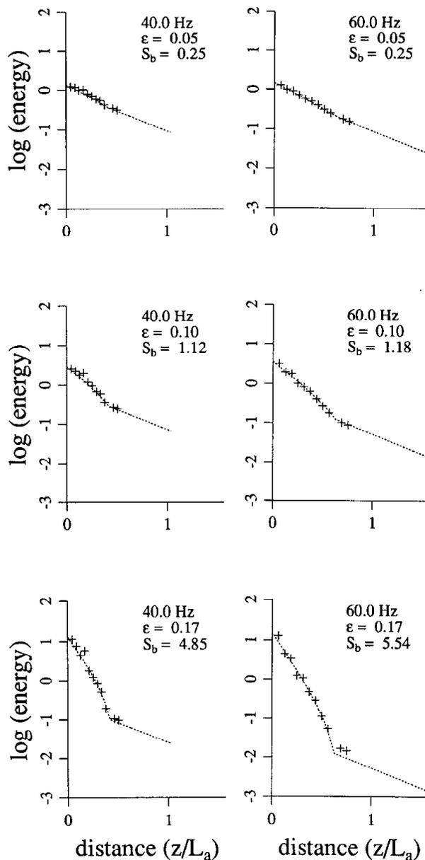
Figure 4: Energy distribution along propagation path in a finite random slab ( $a = 5$  m) for different frequencies with  $2/3$  pass-band averaging. The thickness of the slab is 1 km. The background velocity jumps from 3 km/s to 4 km/s at the bottom of the slab. The crosses are the measured values averaged over 10 realizations and the dotted lines are the theoretical predictions. The top, middle and bottom figures are for weak, intermediate and strong scatterings, respectively.
