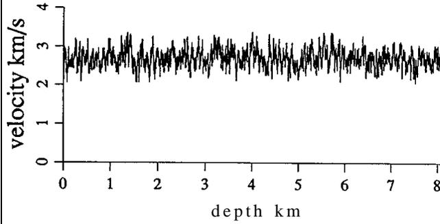
Figure 1: Velocity model of a 1D random medium having mean velocity of 3 km/s, RMS velocity perturbation  $\epsilon = 10\%$  and exponential correlation function with correlation length  $a = 5$  m.
