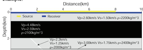
Figure 6. A simple salt layer model with two subsalt reflectors: A steep ( $45^\circ$ ) fault and a flat baseline reflector. The source and receiver distributions on the surface are also sketched.
