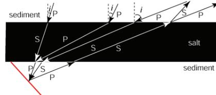
Figure 3. A schematic diagram of converted wave paths that provide illumination to a 45°-dip subsalt fault.
