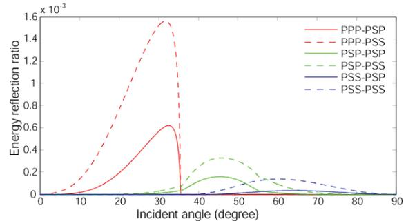
Figure 4. Path efficiency as a function of incident angle for steep fault illumination as shown in Figure 3.
