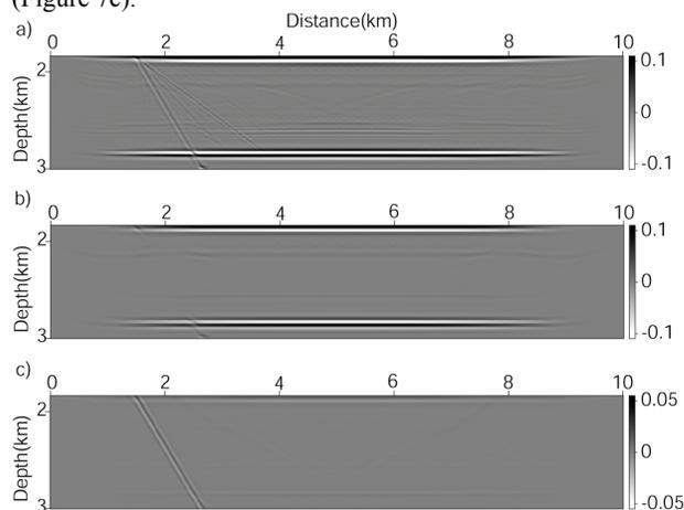
Figure 7. Comparison of a) conventional elastic migration (RTM) (top panel), b) P-P migration (mid panel), and c) the C-path migration using PSP-PPP and PPP-PSP paths (bottom panel). On the panels only the subsalt part of image is shown.
