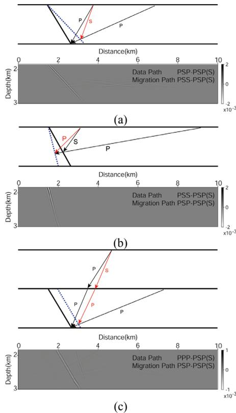
Figure 8. Examples of path mismatch between the data and the migration operator.
