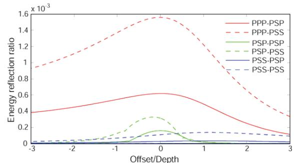
Figure 5. Path efficiency as a function of offset (normalized by reflector depth) for steep fault illumination as shown in Figure 3.
