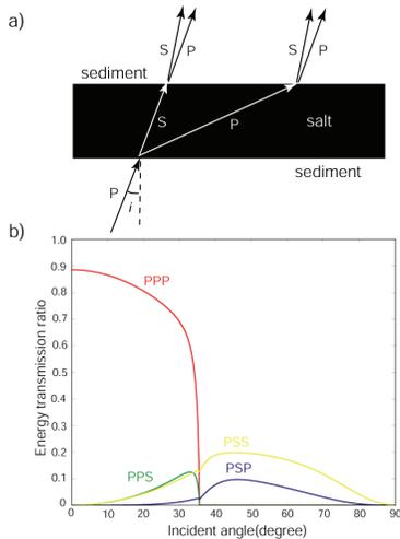
Figure 2. a) A schematic diagram of one-way transmitted wave paths penetrating through a salt layer. b) Energy transmission coefficients for different wave paths.
