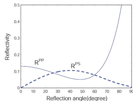
Figure 1. P-P (solid line) and P-S (dashed line) reflectivity on a reflector (fault). Note that at small reflection angles (the angle between the incident direction and the reflector normal), e.g., near normal incidence, the P-to-S reflectivity (conversion coefficient) is very weak in comparison with P-P reflectivity.
