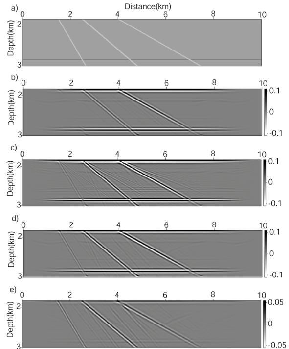
Figure 9 a) The velocity model; ; b) Migrated image with only pure P-path for the whole model; c) Switching on all the wave paths during migration but apply only the P-P imaging condition at the subsalt region; d) Migrated image with PPP-PSP and PSP-PPP path combination.
