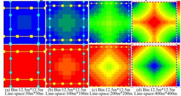
Figure 4: Variations of offset coverage related to the source-receiver line-space. Top: minimum and bottom: maximum offset distributions.
