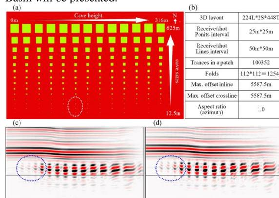
Figure 1: (a) A depth slice for a synthetic model with caves of different sizes. (b) Acquisition and image parameters. (c) and (d) Images using 25\*25 and 12.5\*12.5 m bin sizes.
