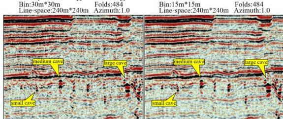
Figure 2: 3D PSDM profiles with different bin sizes
