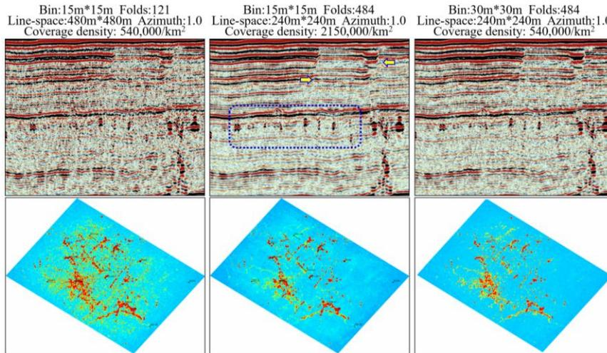
Figure 7: Comparisons of real data imaging with different 3D layouts
