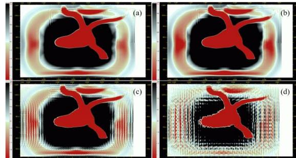
Figure 5: PSDM depth slices for a synthetic river sand body, (a) to (d) are correlated to line-spaces shown in Fig. 4
