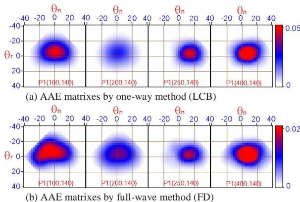
Figure 7, Comparison of the AAE matrix for selected points by one-way method and full-wave method
