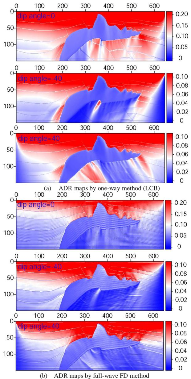
Figure 4, Comparison of the ADR maps for dip angle  $-40^\circ$ ,  $0^\circ$  and  $40^\circ$  by one-way method and full-wave method
