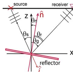
Figure 1, Definition of dip angle and reflection angle
