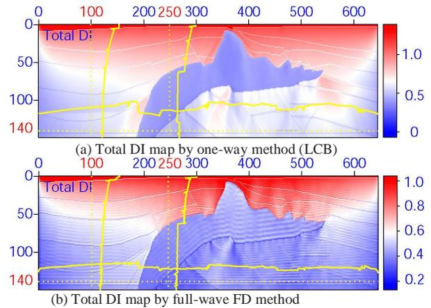
Figure 2. Comparison of the total DI maps by one-way method and full-wave method
