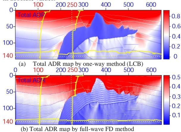
Figure 3, Comparison of the total ADR maps by one-way method and full-wave method
