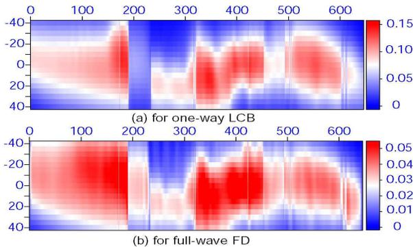
Figure 6, Comparison of the ADR amplitudes along horizontal line 140 for all dip angles.
