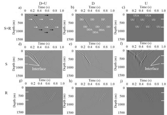
Figure 2. Migrated source and receiver wavefields in  $(z, t)$  domain. Top row: overlapped source and receiver waves, middle row: source waves, and bottom row: time-reversed receiver waves. Left column: total wavefield, middle column: decomposed down-going waves, and right column: decomposed up-going waves.
