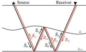
Figure 1. Cartoon showing the up- and down-going sections of source and receiver waves. The black path indicates the forward propagated wave from a source to a receiver and the red path indicates the back propagated wave from a receiver to a source. The arrows indicate the related up- and down-going source and receiver waves.
