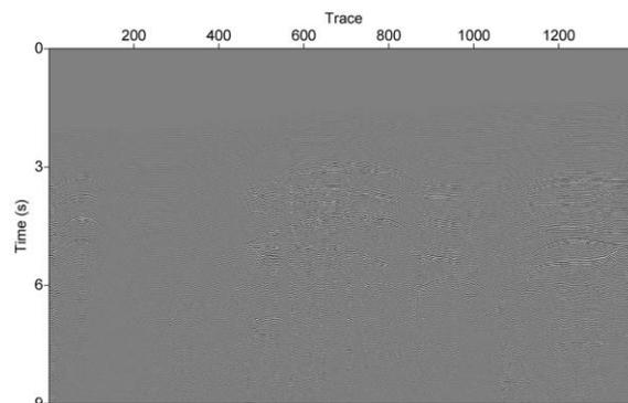
Figure 6. Zero-offset profile by stacking 1387 internal multiple shot gathers
