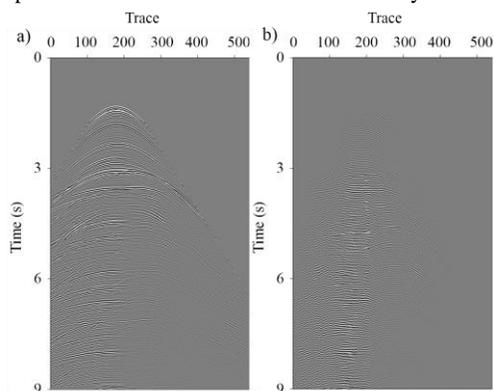
Figure 5. A typical shot gather for SMARRT data set. Left: traces with mixed primary reflections, surface related multiples and internal multiples. Right: predicted internal multiples, where surface related multiples have been removed.
