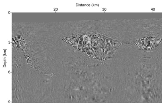
Figure 7. Prestack RTM image from internal multiple only data.
