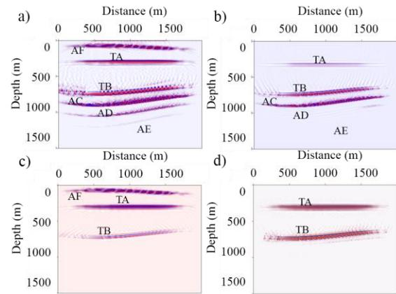
Figure 4. (a) Images from internal multiples without artifact attenuation; (b) UU image with internal multiples; (c) DD image with internal multiples; and (d) the final image from internal multiples after attenuating artifacts.
