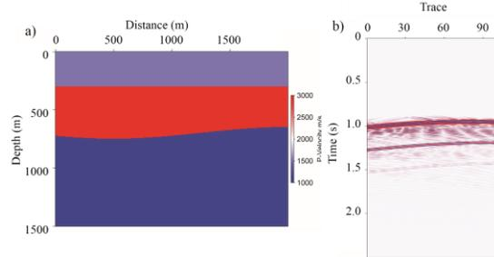
Figure 3. (a) A three-layer velocity model separated by a flat upper interface and a curved lower interface. (b) The common shot record with primary reflections eliminated, where internal multiples up to the third order can be identified.
