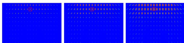
Figure 6: The wavenumber spectra achieved from the PSFs in Figure 4 by Fourier transform. Left: 16 Hz; middle: 24 Hz; and right: 32 Hz.
