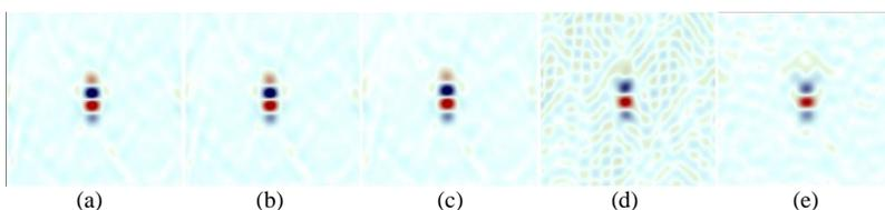
Figure 8: The zoomed in PSFs of different receiver intervals: (a) 5m; (b) 10m; (c) 20m; (d) 40m; and (e) 50m.
