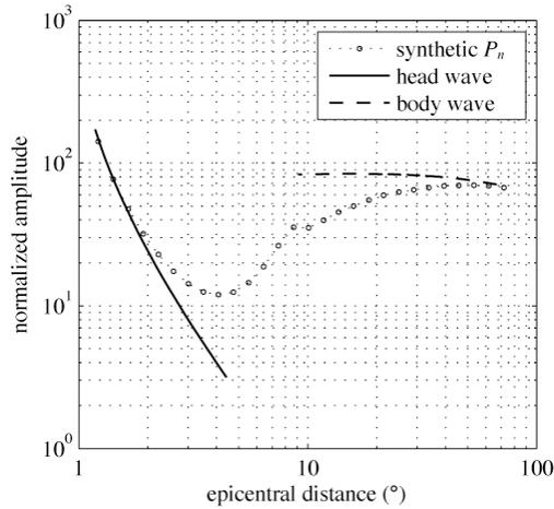
**Figure 2. 10-Hz synthetic  $P_n$  amplitude decay in a spherical Earth model with constant mantle velocities. The solid line depicts the theoretical amplitude decay of a conical head wave in a plane one-layer-over-half-space Earth model. The dashed line is the amplitude decay of infinite-frequency direct wave in a spherical homogeneous Earth model from ray-tracing calculations.**
