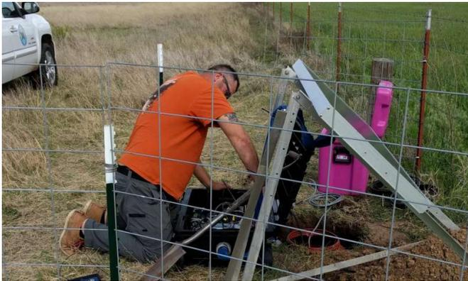
Isaac Woelfel of the Oklahoma Geological Survey installs a temporary seismometer near Quartz Mountain, OK. Scientists continue to evaluate the effects of reductions in wastewater injections on seismic activity in Oklahoma. Credit: Jacob Walter, OGS
