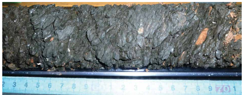
Figure 4. Photo of Core 17 recovered from JFAST site C0019 showing the highly deformed fault zone material.
