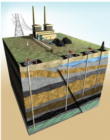
**Small pilot projects are already capturing and storing carbon belowground. A larger-scale system for capturing and storing CO<sub>2</sub> produced by a coal-fired power plant is illustrated above.**
