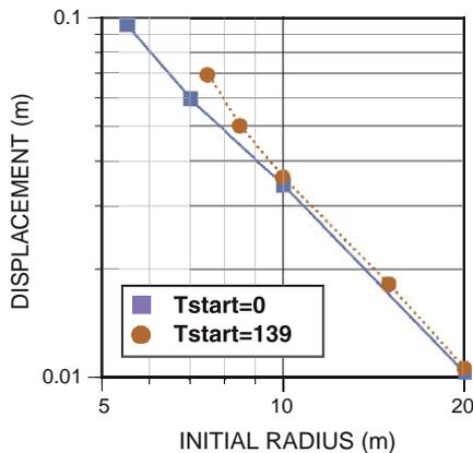
Fig. 6. Displacement after 256 days of motion vs. initial radius, starting either at zero or 139 days.
