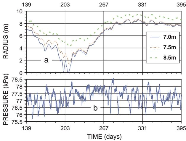
Fig. 5. a) Radius vs. time for three values of initial radius. b) Pressure history, starting at Day 139.
