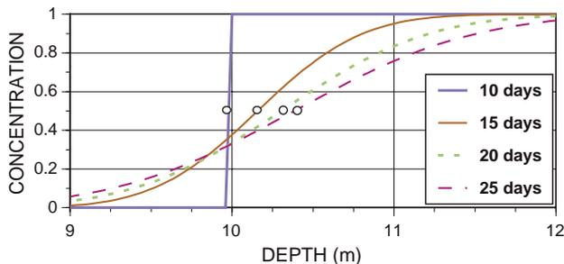
Fig. 1. Profiles of concentration (in relative units) at the end of successive 5-day cycles. Transport started after the flow had achieved steady state at 10 days. Points mark the successive locations of gas with concentration 0.5.
