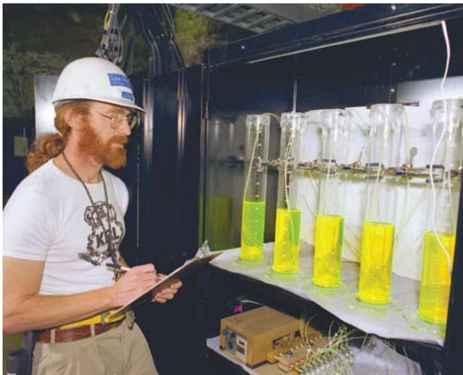
Los Alamos National Laboratory scientist observes injection quantities of traced fluid for the Busted Butte Unsaturated Zone Transport Test.
