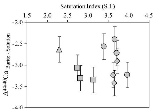
Fig. 8. Synthetic barite results.  $\Delta^{44/40}\text{Ca}_{\text{Barite-solution}}$  vs. Saturation Index (S.I.). Symbols include Experiment 1 (circles), Experiment 2 and 3 (diamonds), Experiment 4 (triangle), and Experiment 5 (squares). Error bars are the average uncertainty = 0.30‰ for the experiments.
