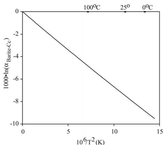
Fig. 5. Theoretical equilibrium  $^{44}\text{Ca}/^{40}\text{Ca}$  fractionation between 25% calcium-substituted barite and calcite,  $1000\ln(\alpha_{\text{Barite-Cc}})$ .
