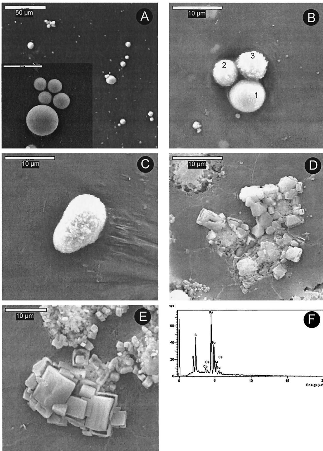
FIG. 1. (A to E) SEM photographs showing the evolution of barite crystals, from initial spherical aggregates to denser barite crystals. (F) Microanalysis of the barite crystal visible in panel D is shown graphically (see text).
