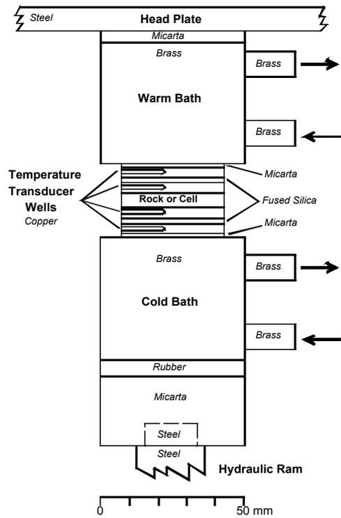
Figure A1. Divided bar method to measure thermal conductivity. The result of such a measurement can clearly be assigned to the direction parallel to the stack axis (after: Pribnow & Sass, 1995).
