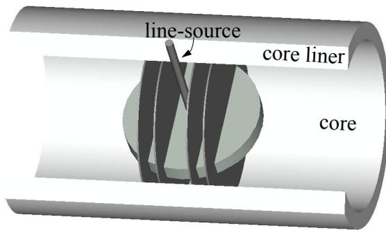
**Figure A2.** Scheme of thermal conductivity measurements with a shipboard line-source. For clarity, the core is not shown and the core liner is cut open. The thin, dark planes represent horizontal bedding in the sediment core. The thick, light-gray disk indicates the plane from which the line-source scans the thermal conductivity. The result of such a measurement is a scalar value composed of horizontal and vertical thermal conductivity components.
