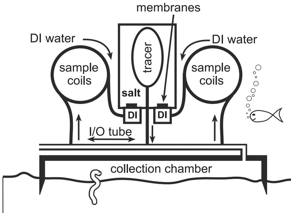
**Figure 3.** Schematic of osmotic seepage meter [after Tryon *et al.*, 2001]. Seepage in or out of the bay floor sediments forces water through the input/output tube. An inert tracer is injected into the I/O tube between two sample coils which draw fluid in from the I/O tube. The magnitude and direction of seepage is determined by the concentration of tracer in the two coils. Tracer injection and suction of water into the sample coils is “powered” by osmotic gradients across membranes.
