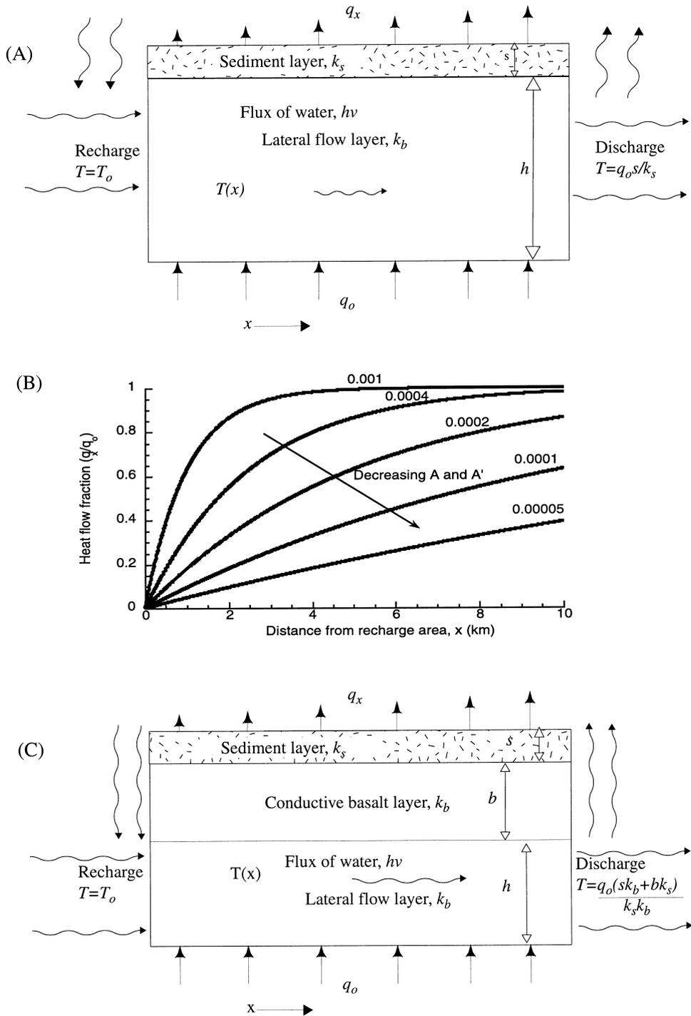
Fig. 1. (A) Cartoon of the WMA model (modified from [9]). (B) Heat flow fraction ( $q_x/q_0$ ) as a function of distance from the recharge area using different values of  $A=k_s/hscvp$ . The same curves apply to the EWMA model using  $A'=(k_b k_s)/(sk_b+bk_s) \cdot (1/hcvp)$  rather than  $A$ . (C) Cartoon of EWMA model.
