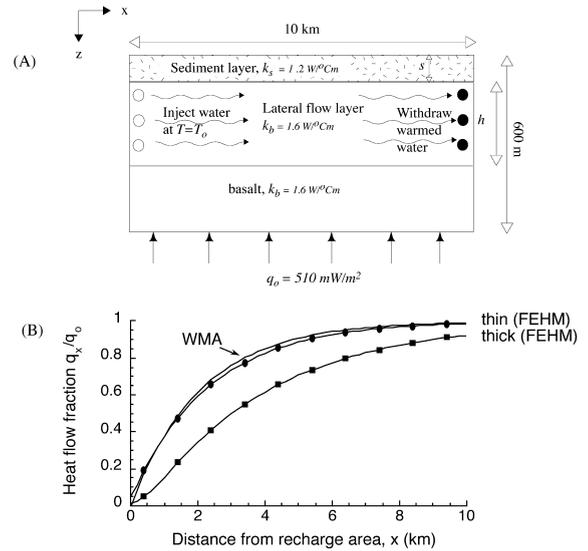
Fig. 3. (A) Model configuration for two-dimensional numerical simulations for partially coupled heat and fluid flow within ocean crust. Grid cells were 200 m (horizontal) by 20 m (vertical). (B) Comparison of analytical and numerical solutions with no vertical mixing. The WMA analytical solution (solid line, no symbols) is identical for the two cases: a thin layer ( $s = 50$  m,  $h = 40$  m,  $\nu = 10^{-7}$  m/s) and a thick layer ( $s = 50$  m,  $h = 400$  m,  $\nu = 10^{-8}$  m/s).
