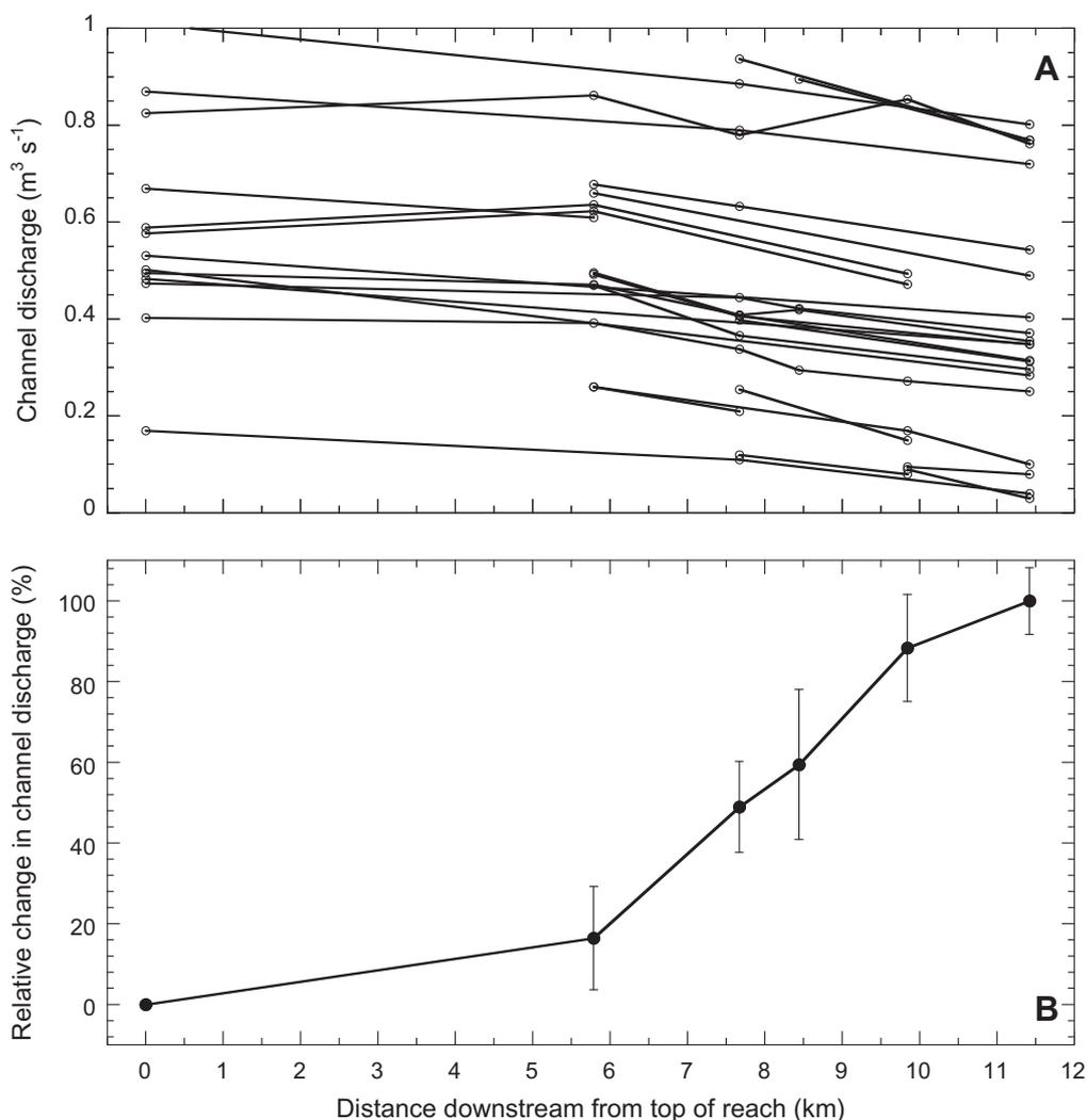
**Fig. 3.** Summary of 32 seepage runs on Pajaro River from 2003 through 2006 along the experimental reach. (A) Individual seepage runs: discharge ( $\text{m}^3 \text{s}^{-1}$ ) versus distance downstream (km). (B) Percentage loss of channel discharge. Error bars indicate standard deviation of measurements.
