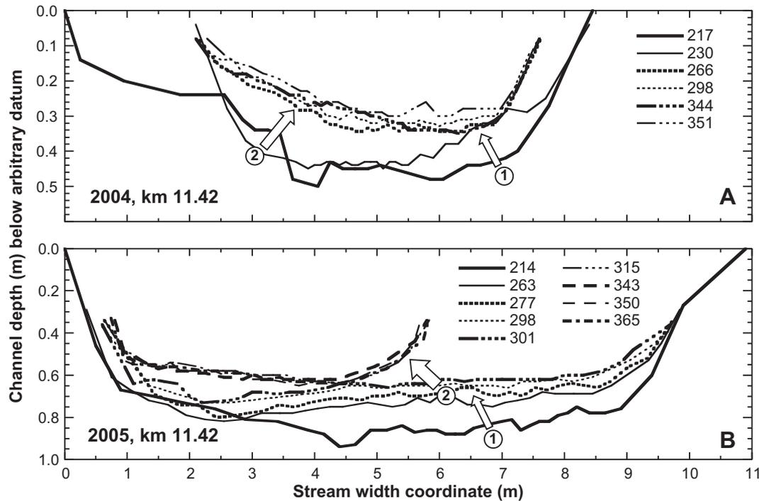
**Fig. 4.** Stream cross-sections of Pajaro River at km 11.42 collected during individual streamflow measurements between May and September on water days indicated (A) in water year 2004 and (B) 2005 illustrate the mobility of the bed sediments and morphologic changes to the streambed at these sites. Arrows indicate the order and evolution of bed shape, and areas of local aggradation and scour ( $\sim 2\times$  vertical exaggeration).
