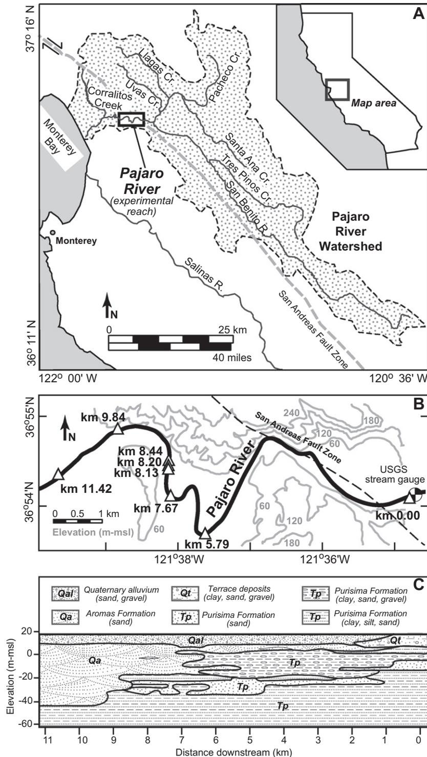
**Fig. 1.** Study setting. (A) Map of the Pajaro River watershed, central coastal California, USA. Inset shows location of experimental reach. (B) Pajaro River experimental reach. Piezometer locations are marked in distances (km) downstream from the USGS stream gauging station (11159000, Pajaro River at Chittenden, CA), km 0.00. (C) Simplified geologic cross section along the Pajaro River experimental reach expanded from compilation of well logs adjacent to river (adapted from Stemler, 2005).
