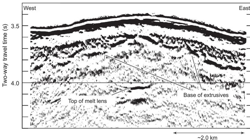
**Figure 3.1** Migrated multichannel seismic profile across the East Pacific Rise at 9°40' N (modified from Harding et al. 1993). Reflectors interpreted to represent the top of a melt lens and the base of the extrusive section are labeled.
