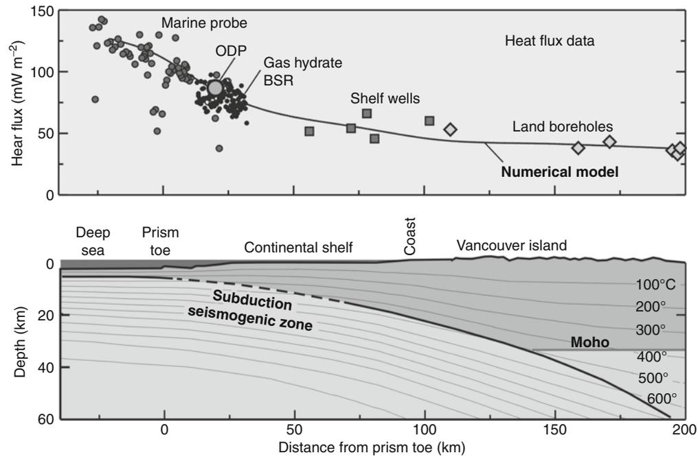
**Seafloor Heat Flow: Methods and Observations, Figure 7** Structural and heat-flux transect across the Cascadia subduction forearc, with temperatures estimated from a numerical model for underthrusting and sediment thickening, constrained by the heat-flux data (following compilation of Hyndman and Wang, 1993).
