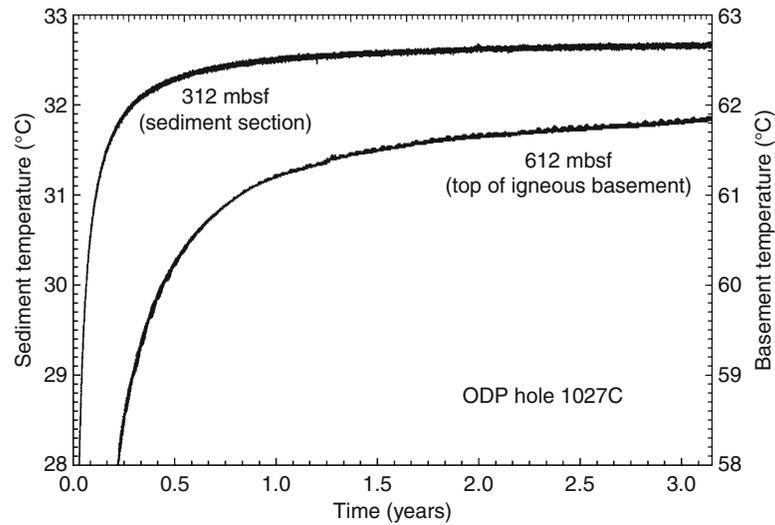
**Seafloor Heat Flow: Methods and Observations, Figure 3** Two records from a 10-thermistor cable suspended in a borehole that penetrates a c. 600-m-thick sediment layer and into the underlying uppermost igneous oceanic crust. The longer recovery time at the deeper level reflects the large volume of water that invaded the uncased and permeable igneous section during the 5 days between the time of drilling and when the hole was sealed and instrumented.
