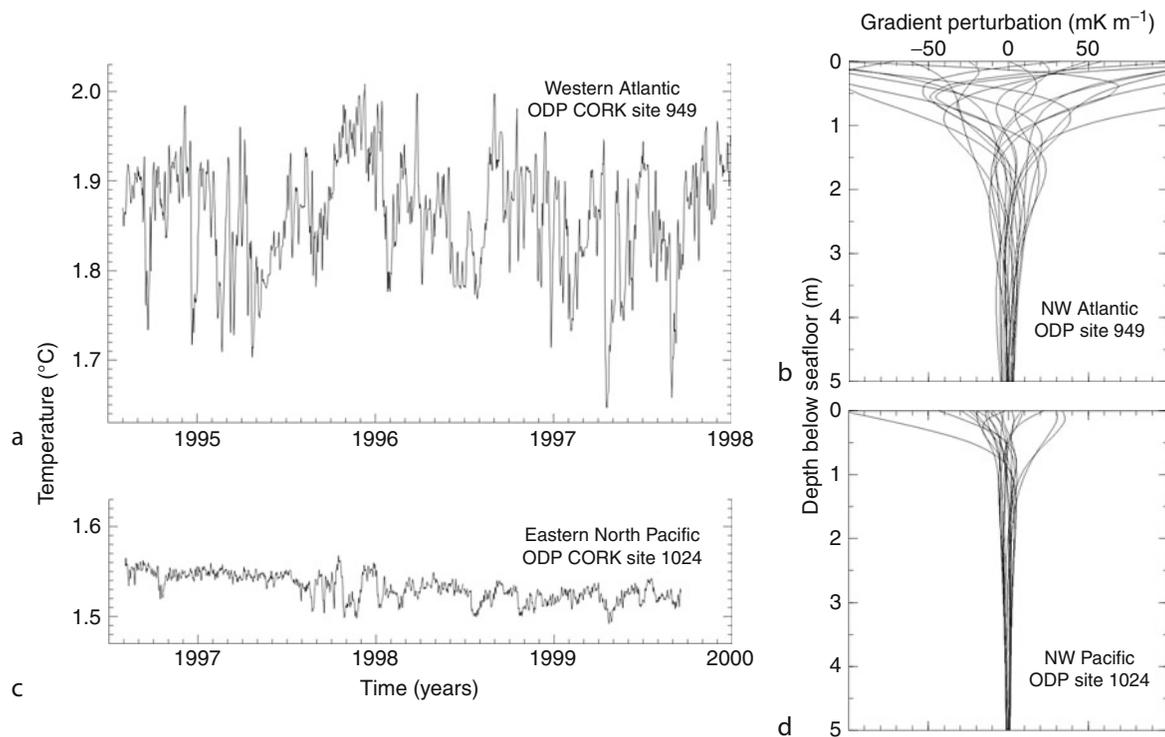
**Seafloor Heat Flow: Methods and Observations, Figure 5** Bottom-water temperature variations observed in the Atlantic (a) and Pacific Oceans (c), and estimated perturbations of the geothermal gradient as a function of depth (b and d) stemming from the variations, calculated at an evenly distributed suite of times during the temperature time series.
