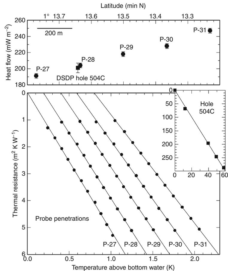
**Seafloor Heat Flow: Methods and Observations, Figure 4** Comparison of collocated seafloor probe and borehole heat-flux observations. Variations in probe measurements along the transect adjacent to the borehole site illustrate how carefully such comparisons must be done.
